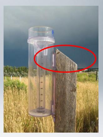
Bevel the top of the post to reduce rain splashing into the gauge
