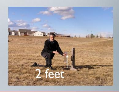
In <u>developed areas</u> place the gauge top approx. 5 feet off the ground
